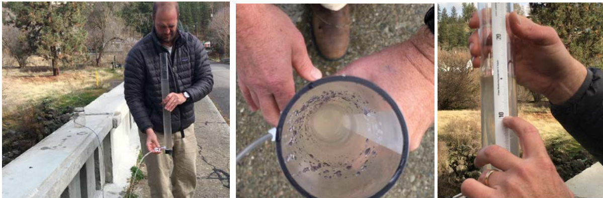
Figure 1. Releasing water until Secchi disc is faintly visible at bottom of tube.
